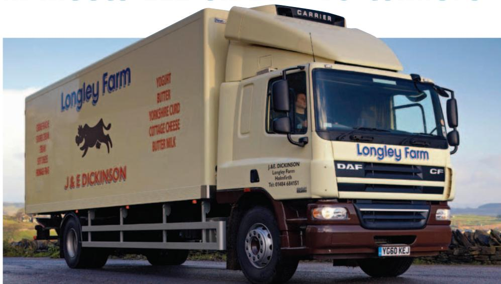
Since their runs involve nights away, both trucks were specified with the DAF sleeper cab, and Paneltex of Hull built and fitted the 53 cubic metre fridge bodies to each of the trucks' 6.9 metre wheelbase.
