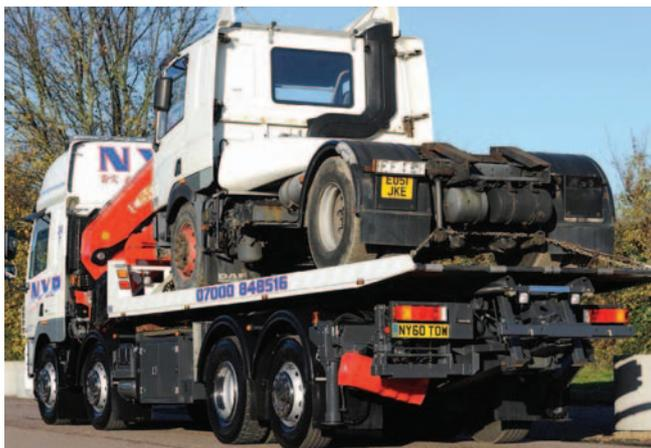
damage-free lifting frame. Other interesting points include a 14,000lb sliding platform winch and extra rear stabiliser jacks – all of which are under remote control, along with the second lift, crane and winch.
